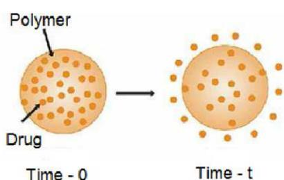
Figure 1 Schematic representation of diffusion across the Matrix
