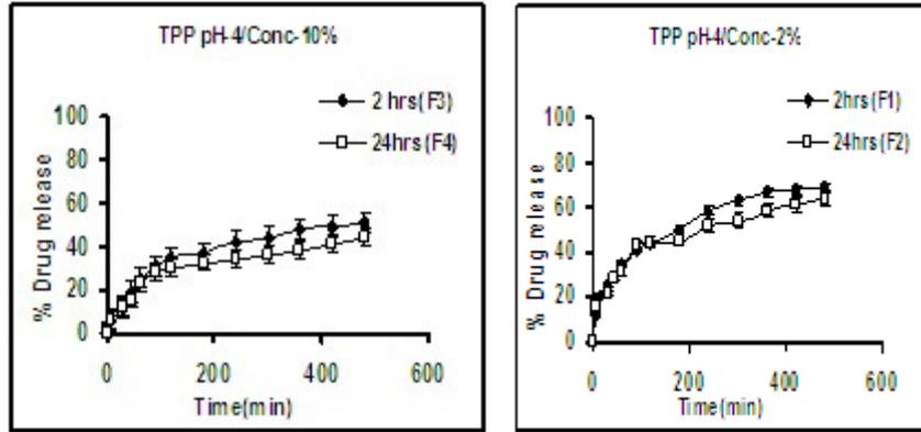
Figure 6: Influence of cross-linking time on the Baclofen release behavior
