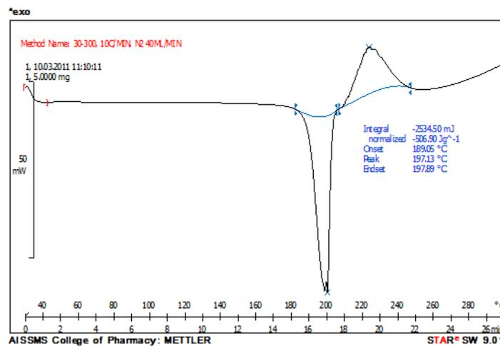
Figure 5: DSC thermo gram drug loaded Chitosan microparticles
