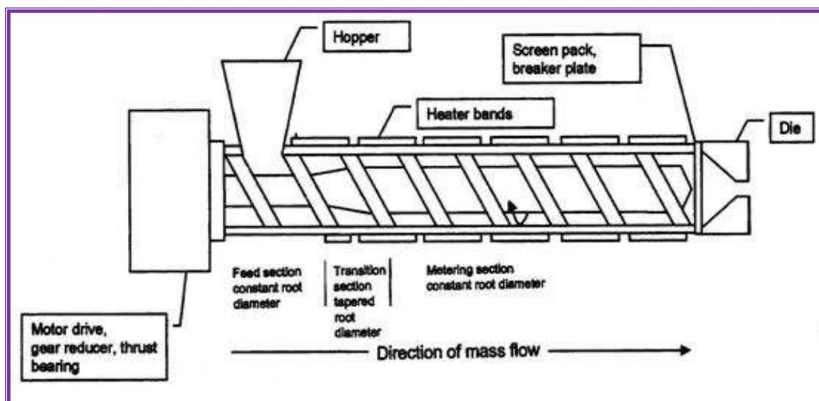
In hot melt extrusion method firstly the drug is mixed with carriers in solid form. Then the extruder having heaters melts the mixture. Finally the melt is shaped in to films by the dies.
