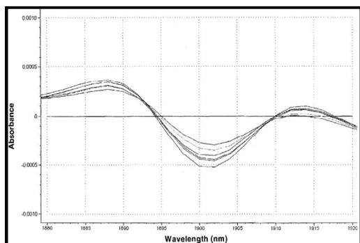
Figure 3: NIR spectra at high, middle, and low positions of a V-blender after 1 minute of mixing.
