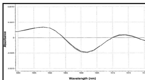
Figure 4: NIR spectra at high, middle, and low positions of a V-blender after 20 minutes of mixing.
