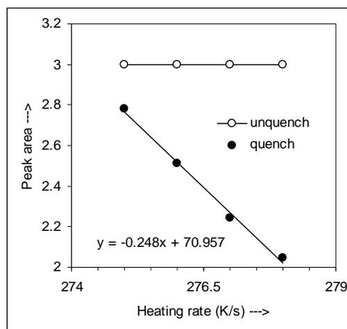
In Figure 5, the behaviour of peak integral (or counts) from equation (4) is shown. The value of  $\Delta T$ 's are 1.31 K, 1.29 K, 1.26 K, 1.25 K for  $\beta = 275$  K/s, 276 K/s, 277 K/s and 278 K/s respectively. The un-quench integral is constant (i.e. peak area is conserved). The quench integral rapidly decreases with increasing heating rates, may be due to the increase of non-radiative recombination. These observations/results may support the theoretical simulation
