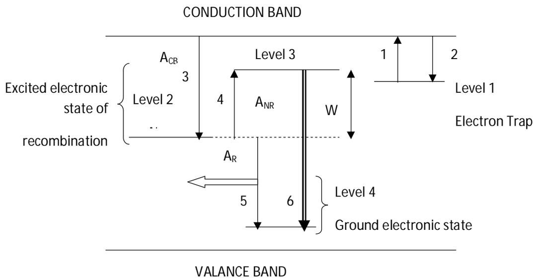
Figure 2: Kinetic model of thermal quenching. Dosimetric trap (Level 1), two excited states within the radiative recombination centre (Level 2 and 3), and the corresponding ground state (Level 4). The various transitions are shown.
