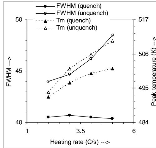
Figure 4: FWHM and peak positions of quench and unquenched glow curves from Figure 3. The relation between peak temperature and heating rate is quadratic, i.e. .
