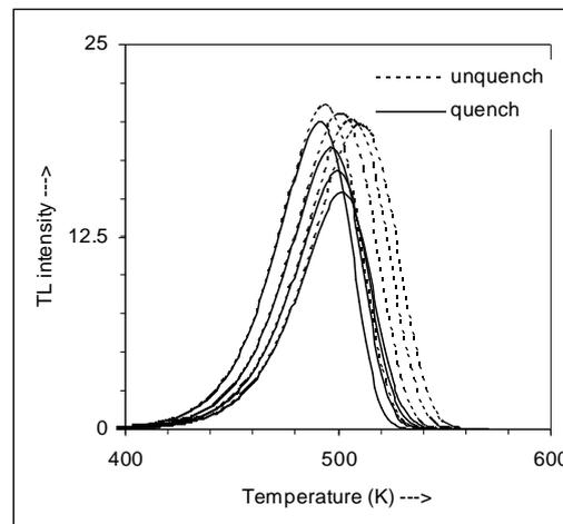
Figure 3: TL glow curves of un-quench and quench. Kinetic parameters for this TL curves were obtained from experimental data.
