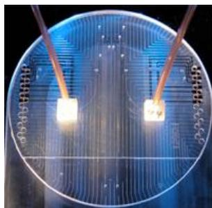
**Figure 1: A top view of a lab on a chip system that is structured on a glass-silicon substrate<sup>[7]</sup>.**
