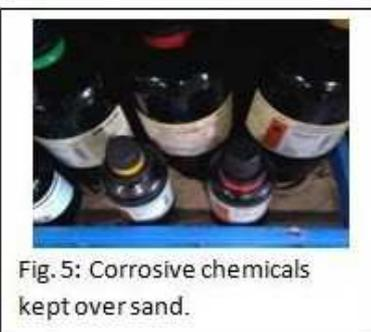
Fig. 5: Corrosive chemicals kept over sand.
