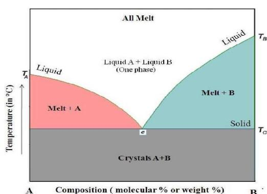
FIG. 1 Phase diagram for a eutectic system
