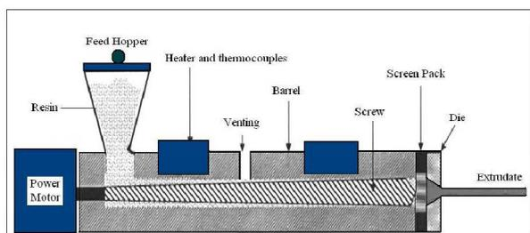
**FIG 7: Schematic showing components of a single screw.**
