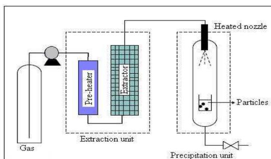
**FIG6: Schematic of the RESS apparatus used in supercritical fluid technology**
