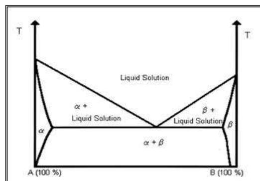
FIG. 2 Phase diagram for a discontinuous solid solution
