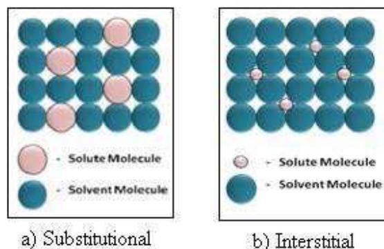
**FIG. 3 Substitutional and Interstitial crystalline solid solution**
