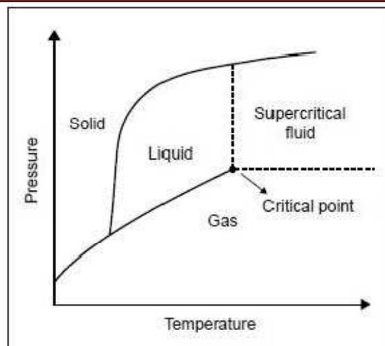
**FIG 5: Supercritical region of a hypothetical compound (Indicated by the dotted lines)**
