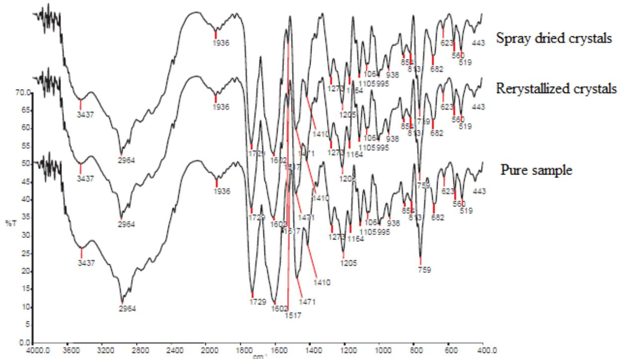
**Fig 2 Shows FT-IR Spectrum of different samples of Valsartan**
