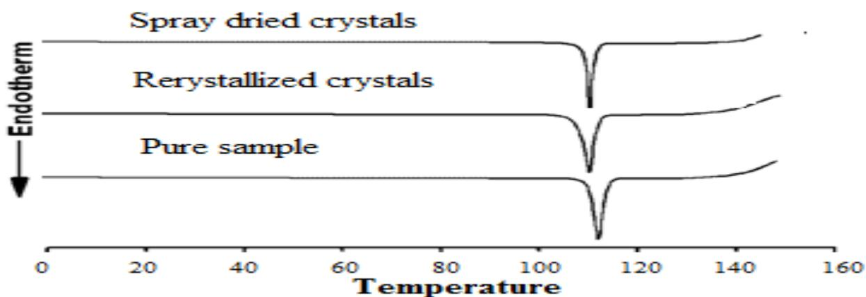
**Fig 1 Shows DSC Spectrum of different samples of Valsartan**
