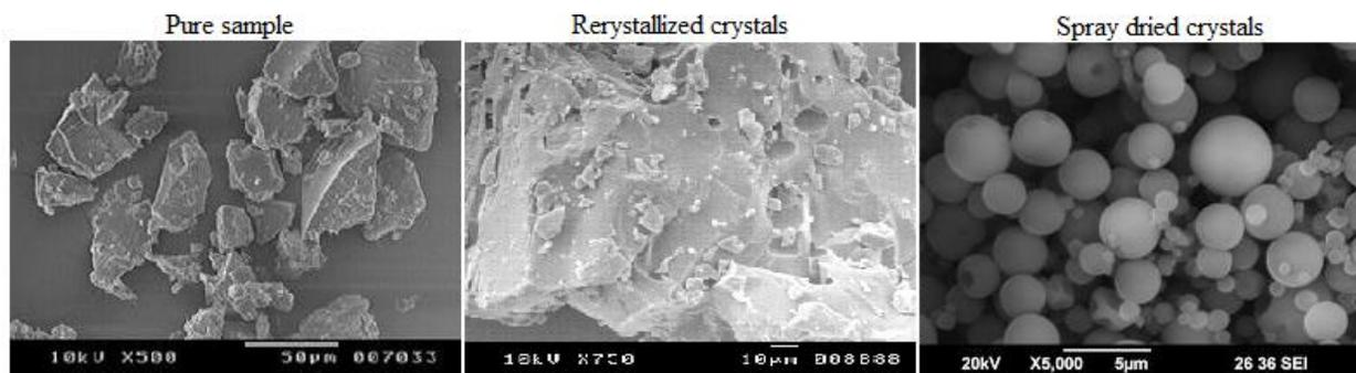
**Fig 4 Shows SEM photographs of different samples of Valsartan**
