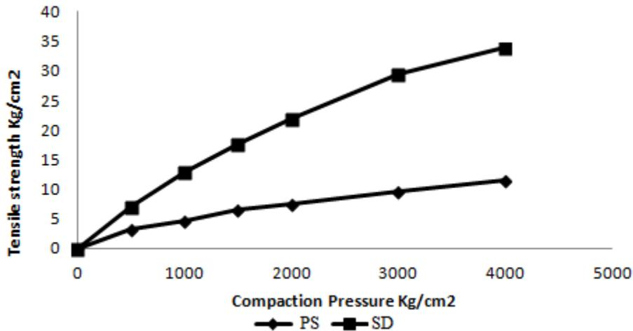
**Fig 5 Tensile strength of different samples of Valsartan**
