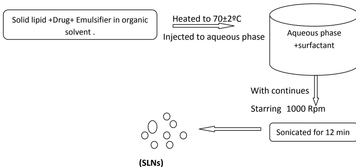
Fig 6: Solvent injection technique
