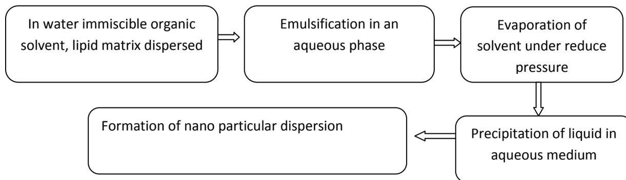
**Fig. 4: Schematic representation Solvent emulsification-diffusion method**
