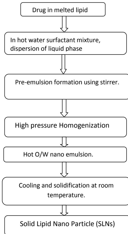
**Fig1: Solid lipid nanoparticles preparation by hot homogenization process.**
