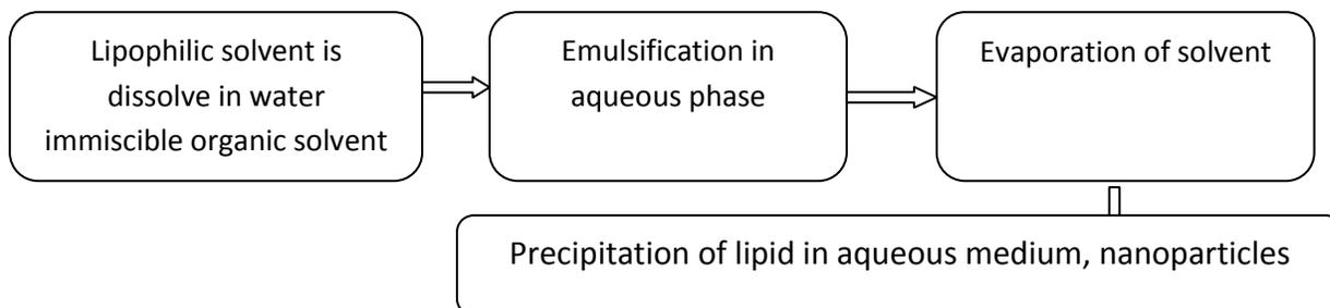
**Fig. 3: Schematic representation of solvent evaporation technique**
