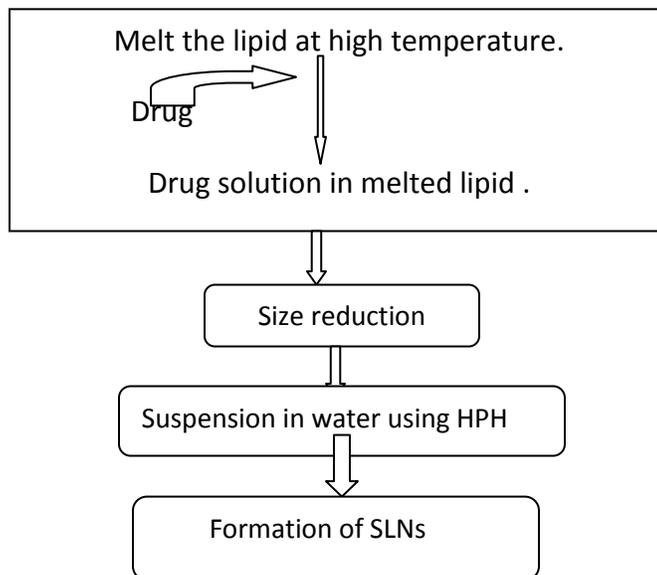
**Fig. 2: Solid lipid nanoparticles preparation by cold homogenization process.**
