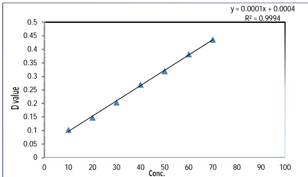
Fig. 4: Calibration curve of Artesunate at 222 nm
