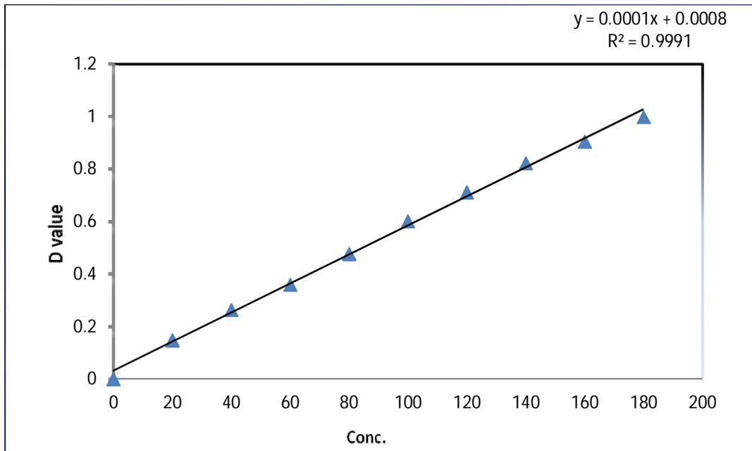
Fig. 6: Calibration curve of Mefloquine at 241 nm
