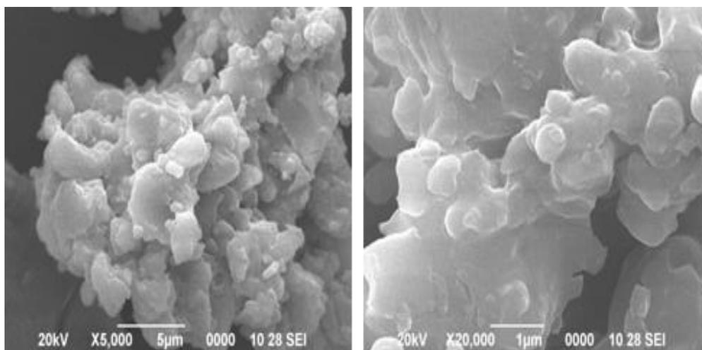
Fig4. Surface morphology of ZnO nanoparticles at different magnifications
