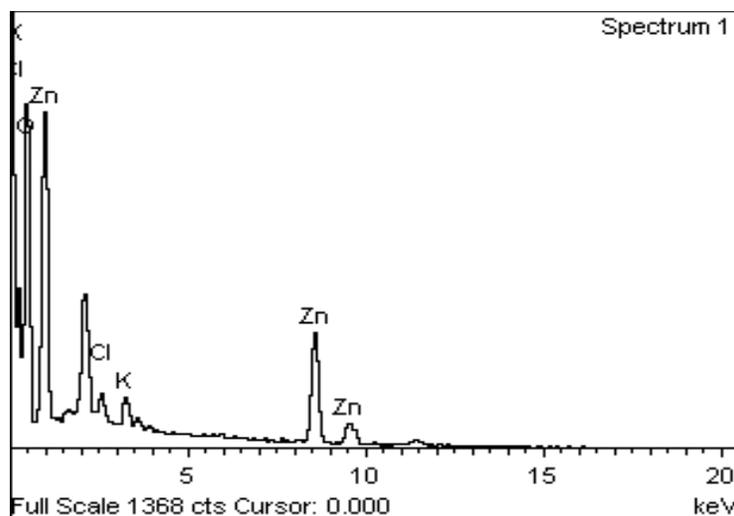
Fig5. EDX images of ZnO nanoparticles
