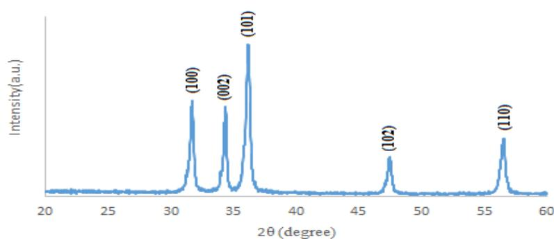
Fig2.XRD pattern of ZnO nanoparticles of heated sample.
