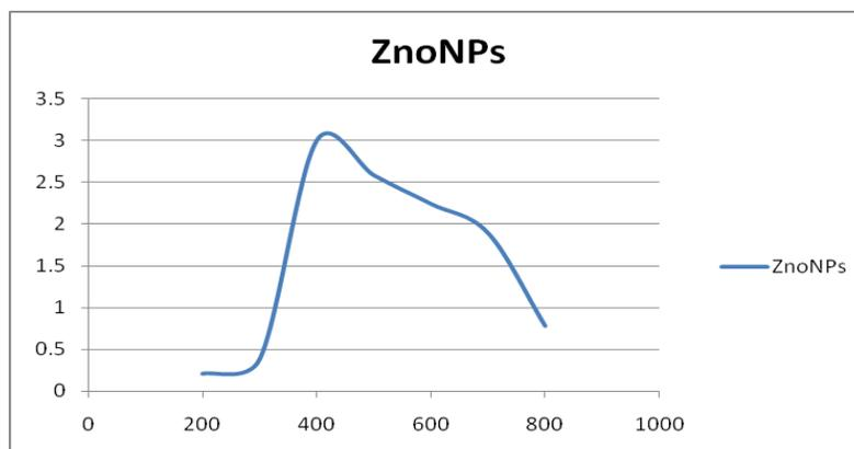
Fig1. UV-Vis spectrum of synthesized ZnO NPs
