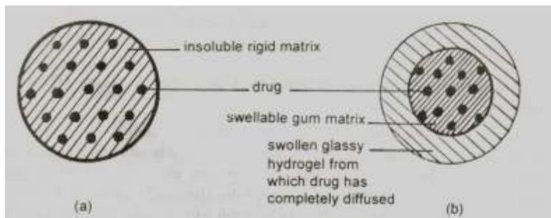
**Fig no.3 Diffusion controlled devices – (a) rigid matrix, and (b) swellable matrix.**
