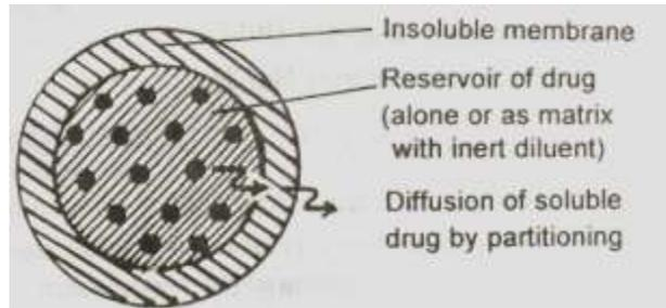
Fig: Drug release of diffusion across the insoluble membrane of reservoir device.
