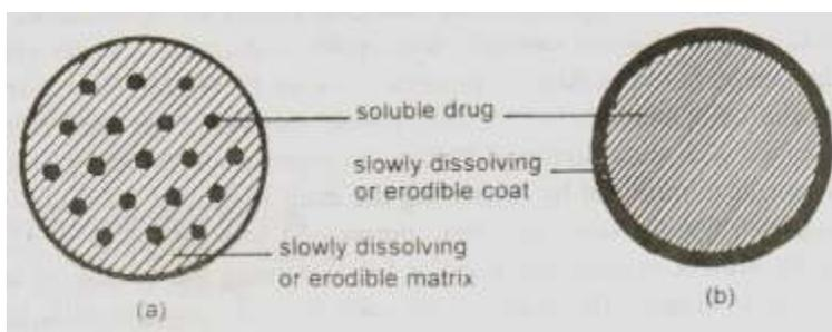
**Fig No.2: Schematic representation of dissolution controlled release systems –(a) matrix system, and (b) coated/encapsulated system.**
