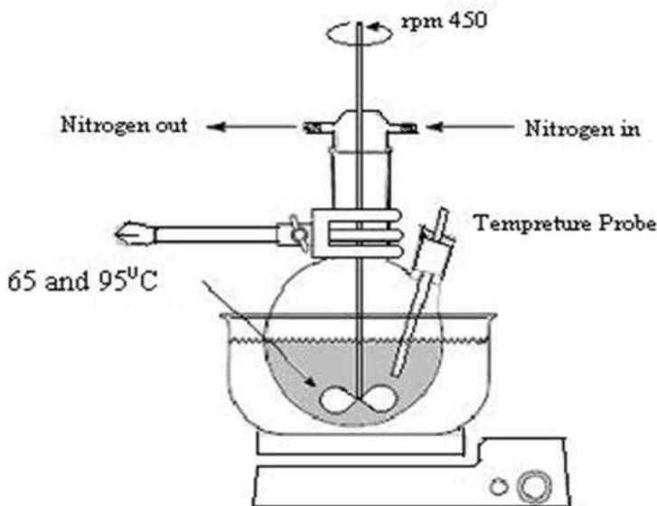
**Fig 2: Reaction vessel for Microspunge Preparation by Liquid-liquid suspension polymerization method.**
