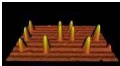
Fig-2: Nano CD: LMR in ASCII encoded in the positions of Nano manipulated 15nm Au particles
